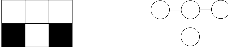
Figure 5.2: A 2D grid map and its graph representation: black cell represents an obstacle, while white cells denote free space.
